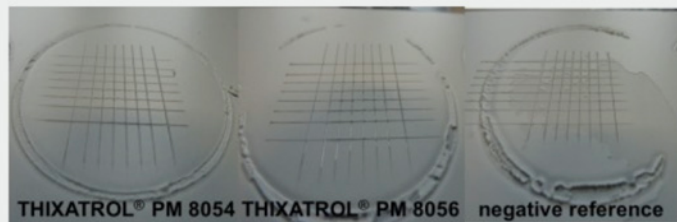
FIGURE 8: Intercoat adhesion testing
